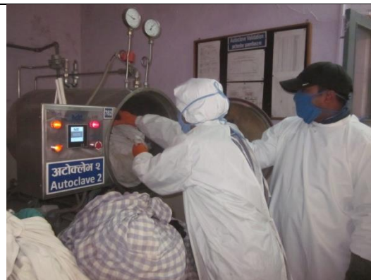
Figure 13. Loading risk waste in the autoclave
